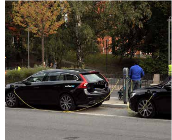
Figure 60: Inset parking with electric vehicle charging points.
